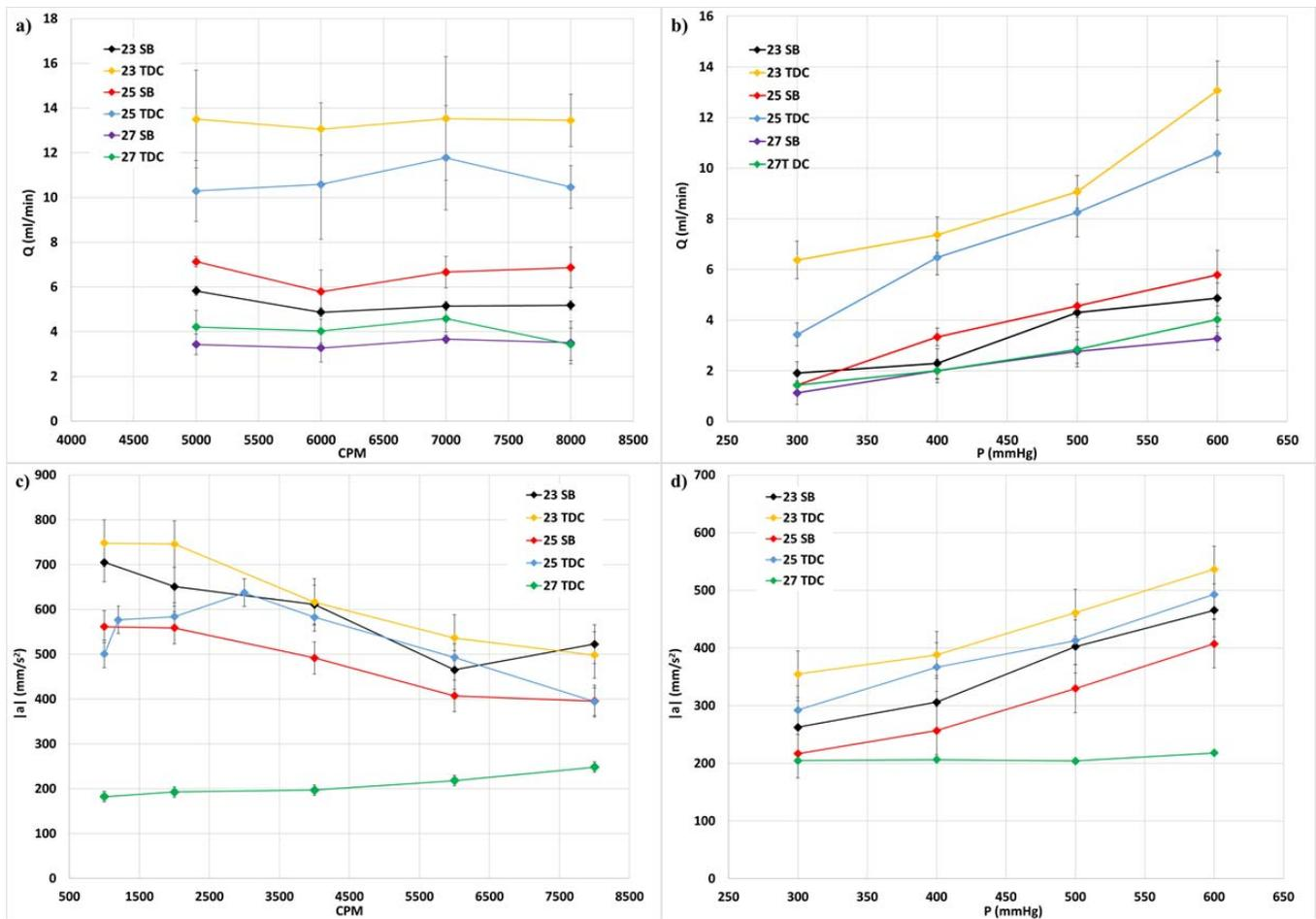
**Figure 7.** Flow rate versus the cutting frequency (a) and the sucking pressure (b). Space and time averaged acceleration versus the cutting frequency (c) and the sucking pressure (d). Experiments in AV.
