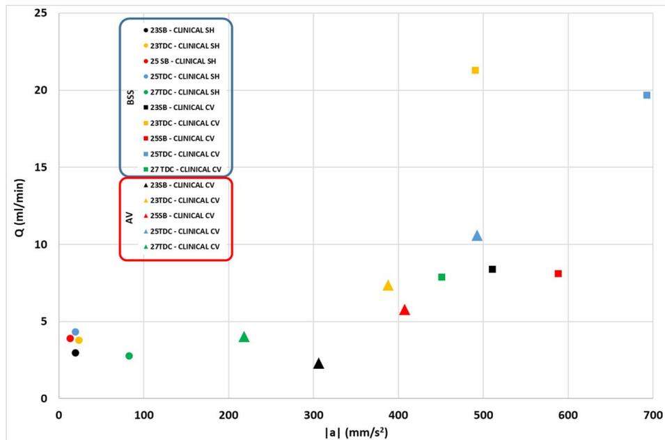
**Figure 8.** Plot of the flow rate,  $Q$ , versus the averaged acceleration  $|a|$  for all tested cutters in BSS and AV. The experiments plotted refer to common clinical settings for each cutter dimension.
