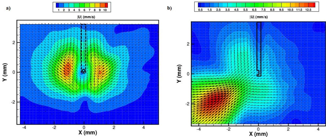
**Figure 5.** Time-averaged maps of velocity magnitude and velocity vectors. The needle is located along the axis  $x=0$  (for  $y > 0$ ) and the port is centered in the point  $x=(0, 0)$ , the position of the cutter is sketched on each map. (a) Front view, (b) lateral view with the cutter port on the negative side of the  $x$ -axis. Twenty-five gauge, TDC, core mode, and 4000 cpm.
